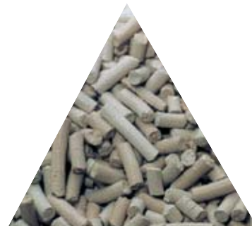
NIAP-02-03, copper-promoted low temperature ZnO absorbent
